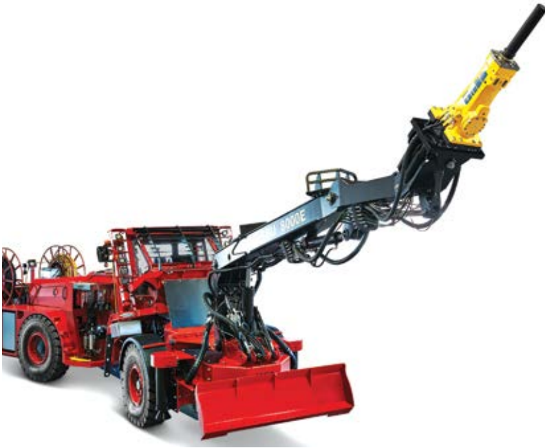
The battery-powered SBU 8000E scaler has a powerful 160-kW electric motor and offers up to 600 Nm of torque. Jama supplies the machine. The battery is rented from Epiroc. (Image: Jama)
