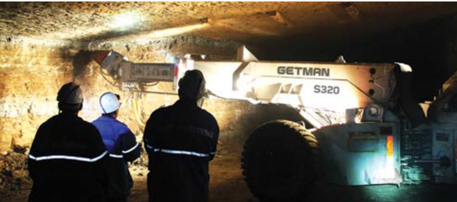
The operator compartment on S300-series scalers is at the far rear of the machine, adding to operator safety. The line of sight to the scaling area offers optimal visibility. (Photo: Getman Corp.)
