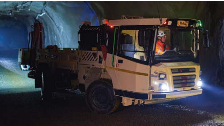
Above, the agile Variomec XS transports materials at the Pyhäsalmi mine in Pyhäjärvi, Finland. XS-series machines have high payload capacities and four-wheel steering. (Photo: Normet)
