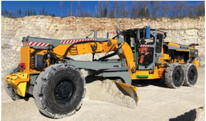
The new GR5 Grader is designed to tear down to fit into shipping crates and hoist cages. It features articulation, and an advanced hydrostatic drivetrain system. (Photo: MacLean Engineering)
