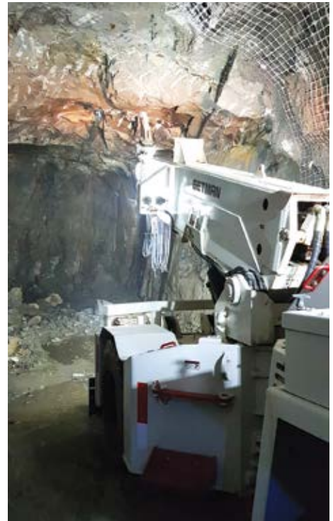
Available boom lengths for S300-series scalers are 6.1 m, 7.3 m and 9.1 m. Available accessory tools on select models include a pick, hammer and rotary cutter. (Photo: Getman Corp.)
