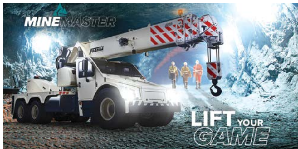
The Minemaster pick-and-carry crane has a compact footprint and is designed for, among other things, lifting and laying pipes, and changing out engines. (Image: Franna)
