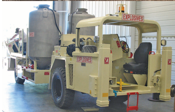
Before and after Getman rebuild of ANFO loader truck
