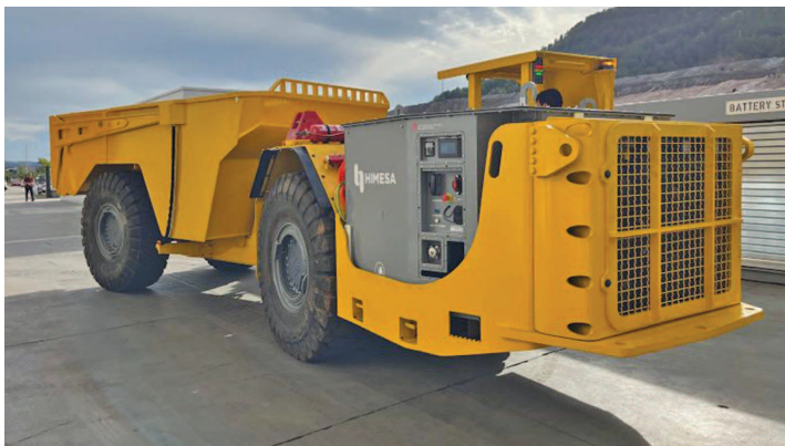
HIMESA battery converted MT2010E from original Epiroc MT2010 Minetruck
