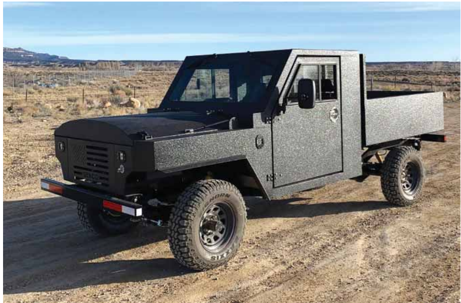
The Small Boss Buggy features a Tier 4-Final engine with streamlined electronics. To facilitate maintenance and cut costs, it has neither a diesel particulate filter nor diesel exhaust fluid. (Photo: Genco)
