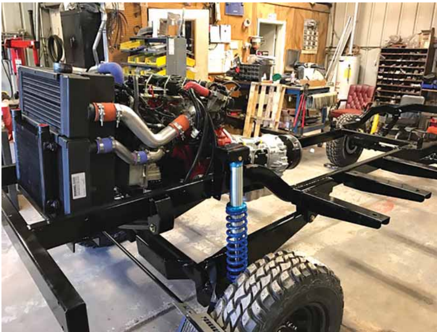
Genco Mine Service co-develops a Cummins Tier 4-Final engine that uses exhaust gas recirculation and diesel oxidation catalyst technologies. The engine is simple and easy to maintain. (Photo: Genco Mine Service)
