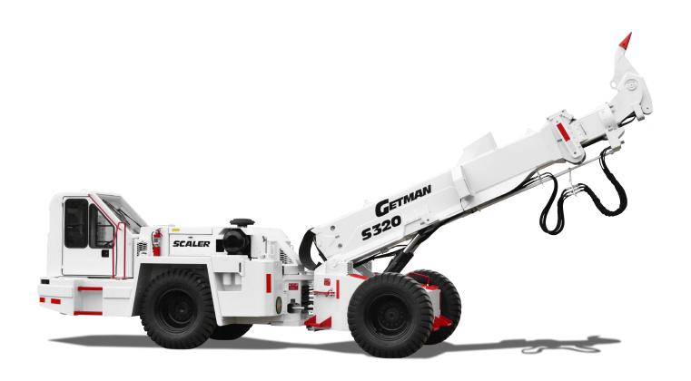
Getman mechanical scalers are a key component of maintaining safe and productive working environments in underground operations, performing the necessary task of scaling safely and effectively through a purpose-built design philosophy. Mechanical scaling is the safest way to bring down loose material from back and rib surfaces.
