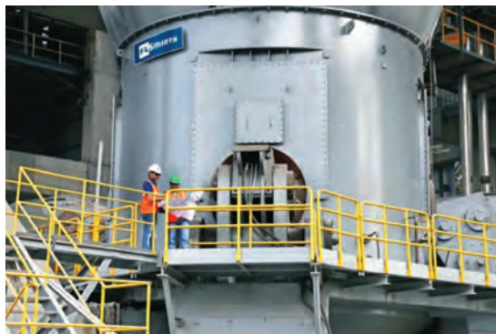
FLS options for dry grinding include Vertical Roller Mills
