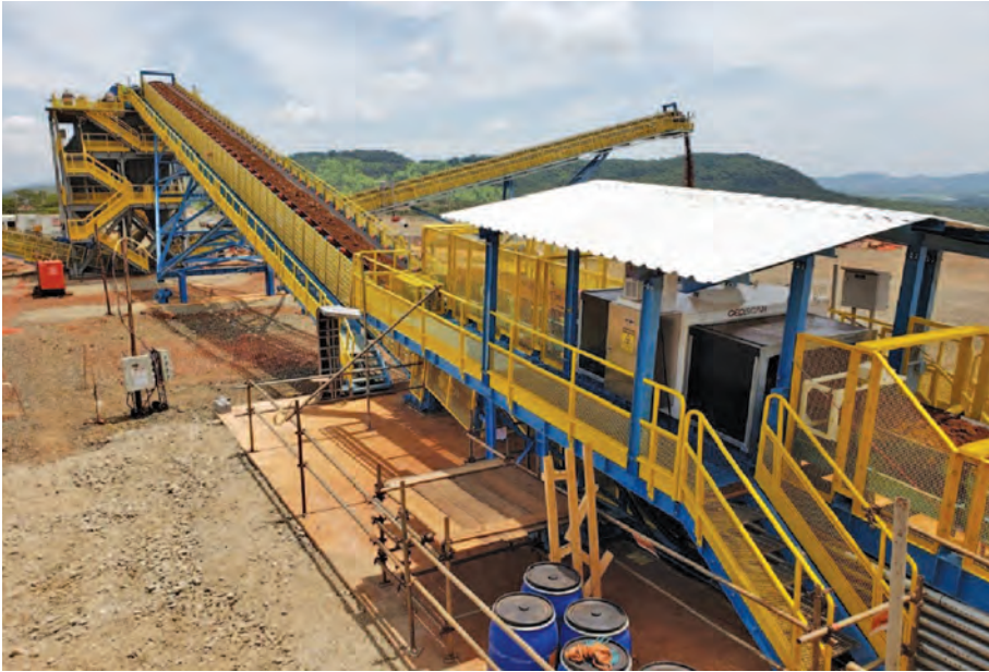
GEOSCAN GOLD specification analyser measuring each 30 seconds of conveyed flow for bulk ore diversion
