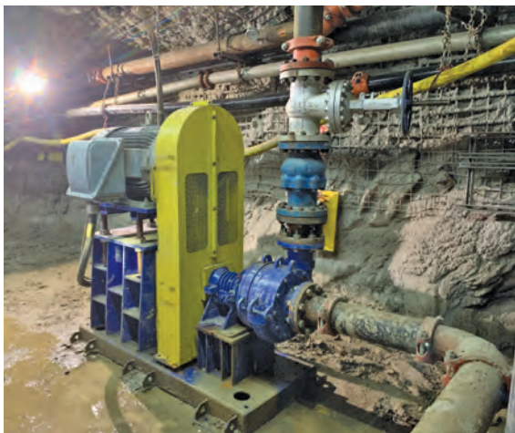
Warman® DWU 75 single-stage high-pressure pump, ensuring uninterrupted mining production in an underground operation
