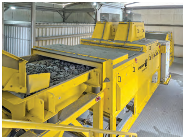
At Ferbasa, the use of STEINERT SBS technology has enabled an increase in production, in addition to reducing costs in the subsequent processes, such as comminution and the use of inputs (reagents)
