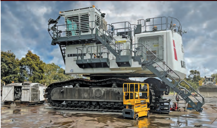
In 2023, Liebherr Mining achieved its first repower of a diesel-drive machine to electric drive, converting a R 9400 in Australia for Fortescue
