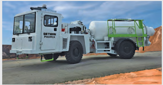
Getman's new ProMix 6 features a horizontal drum mixer with 4.6 m 3 concrete transport capacity
