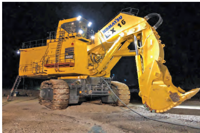
A PC8000 converted from diesel to electric in Zambia
