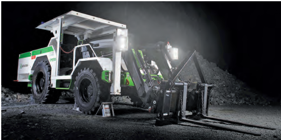
A Kovatera application for material handling based on the Kovatera KM200 tractor
