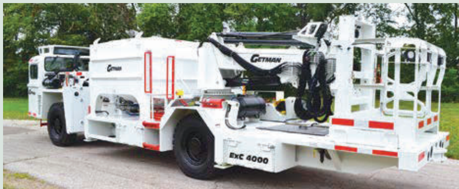
The ProCharge Emulsion MAXX Integrated Emulsion system for the ExC 4000 explosive charger includes the emulsion, water, gasser tanks and a hose handling system. (Photo: Getman Corp.)
