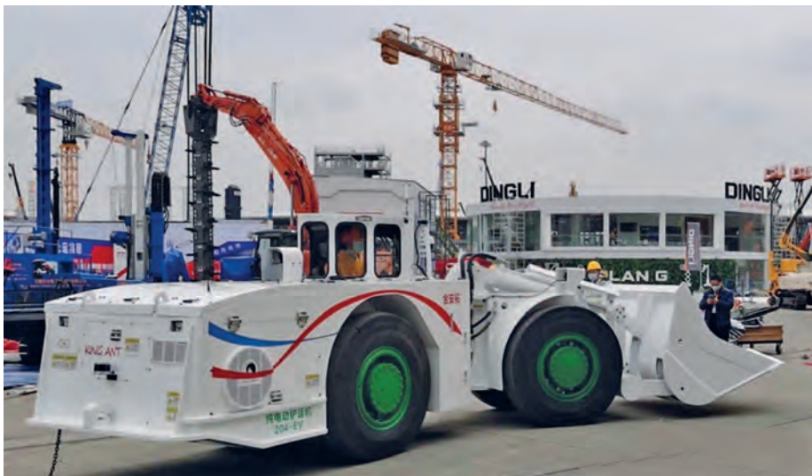
JCHX all lithium battery electric 2 m 3 underground LHD at Bauma China in Shanghai.
